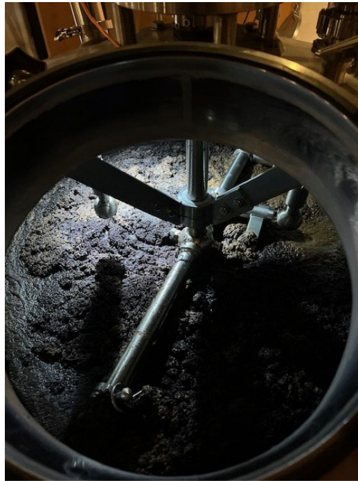
Picture 1 – Notice Loading Level and Dry Bed
